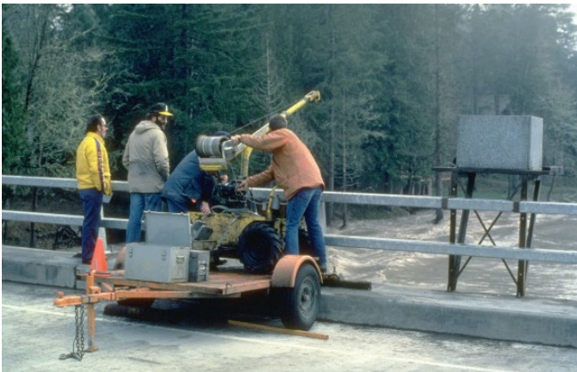
Sediment sampling on the Toutle River at Tower Road during a flood. Dick Jesser is second from the left. (December 12, 1982)
