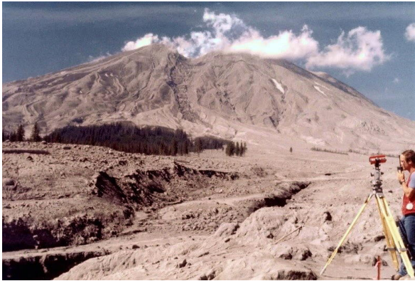
Mike Nolan surveying a channel cross-section on the Pine Creek–Muddy River fan, a surface on the lower SE flank of the volcano that was swept by a large, high-velocity (45 mph) lahar during the first few minutes of the May 18 eruption. The Shoestring Glacier, visible below the notch in the crater rim, was scoured locally more than 30 feet by pyroclastic flows, which provided the meltwater for the lahar (Summer 1980).
