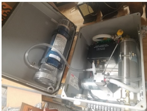
A Sutron Accububble bubbler system. This (and a couple of other makes/models) replaced nitrogen tanks, Cono flow site-feed systems, and mercury manometers. Equipment employs air pump and precisely regulates forward pressure through a bubbler line and orifice, and senses back-pressure changes to recognize direction and magnitude of water-level changes.
